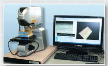
Laser microscope for measuring shapes
