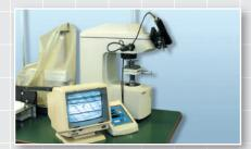
Tester for measuring micro hardness
